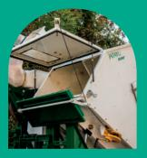
JATAYU Super has a large storage capacity as it is equipped with a hydraulically adjustable 1.5 m<sup>3</sup> Aluminum Hopper container which has a load-bearing capacity of ONE ton.
