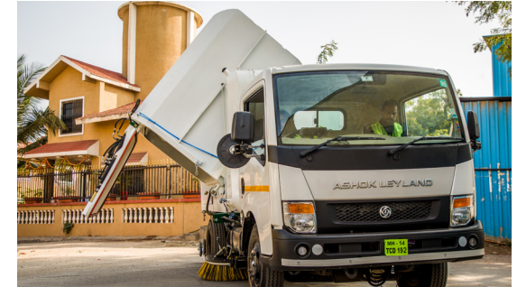
Quick Mid-Dump Hopper Design for Faster Turnaround.
