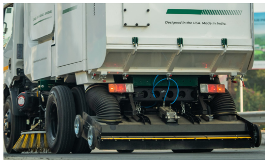
Rear Engine and Rear Head for Ease of Maintenance.
